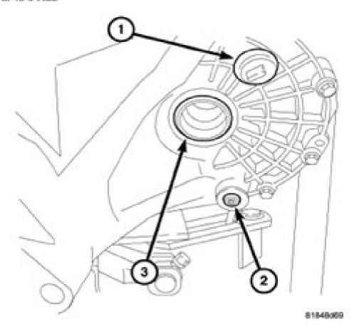
NOTE: All T355 Manual Transactes require the use of ATF+4 (Automatic Transmission Fluid).
