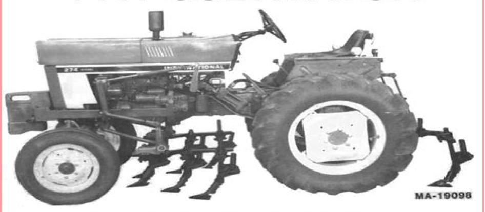
Cultivator on tractor 616 tool equipment and optional rear section shown
