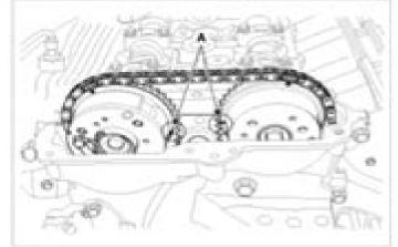
Mark the timing chains (A) corresponding to the timing me
