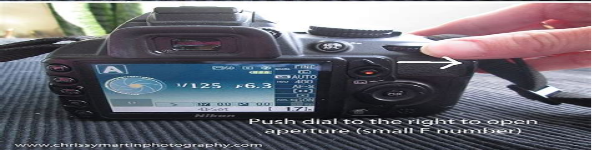
Push dial to the left to open aperture (small F number)
