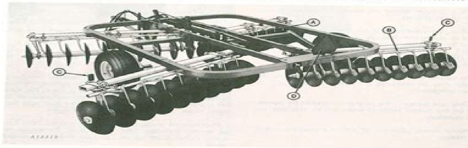
C—Reflector D—Slow Moving Vehicle Emblem
