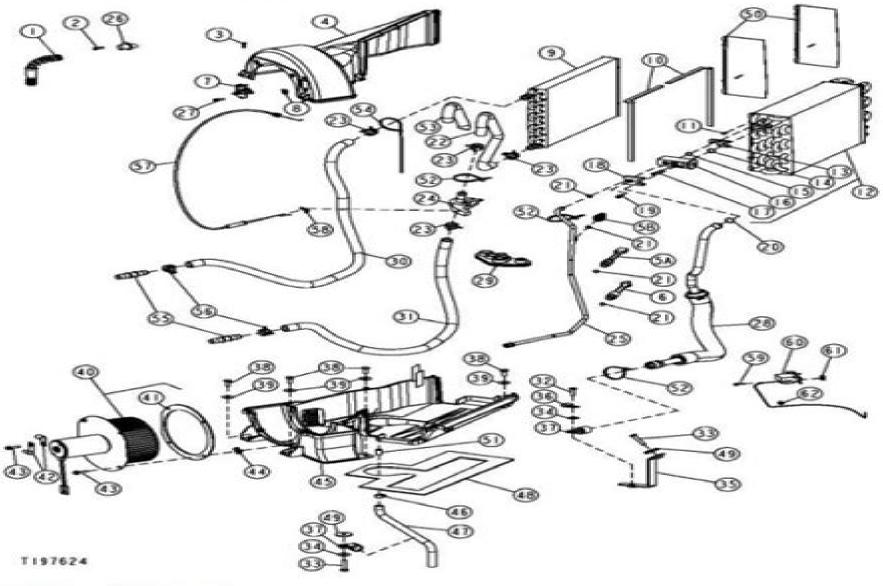
Heater Core and A/C Evaporator
