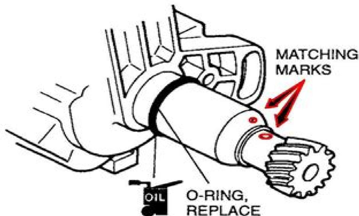
Fig. 1: Camshaft/Distributor Matching Marks
