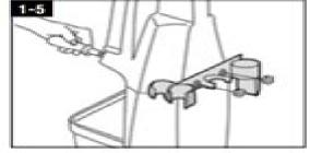
Place nuts in recessed areas on back of handle. Hold each nut in place while tightening each bolt securely (from the front of the handle) with a Phillips screw driver.
