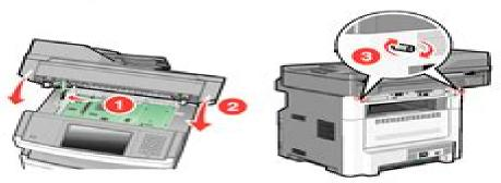
Warning—Potential Damage: Make sure the system board is locked to prevent possible damage to the printer if it is moved.
