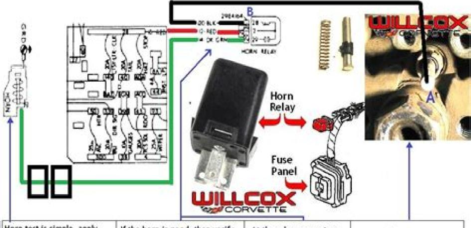
Horn test is simple, apply direct 12 volts to the horn. If the horn blows its good, if not then run a ground jumper from horn case to ground and apply 12 volts again. If horn blows, remove and clean ground brace, reinstall. if the horn is good, then verify continuity from the green horn wire to the relay connector under the dash. If good then test the red wire for 12 volts. If no continuity exist then check bulk head connection or find the break in the wire.
