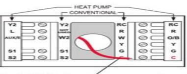
For 24VAC primary power, connect common side of transformer to "C" terminal.
