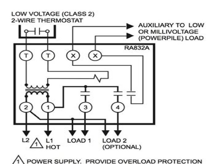
Fig. 3. Internal schematic and typical hookup for RA832A.
