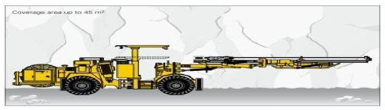
Hydraulically controlled mining and tunnelling face drilling rig with two BUT 28 booms. Available with a variety of rock drills to suit customer requirements.
