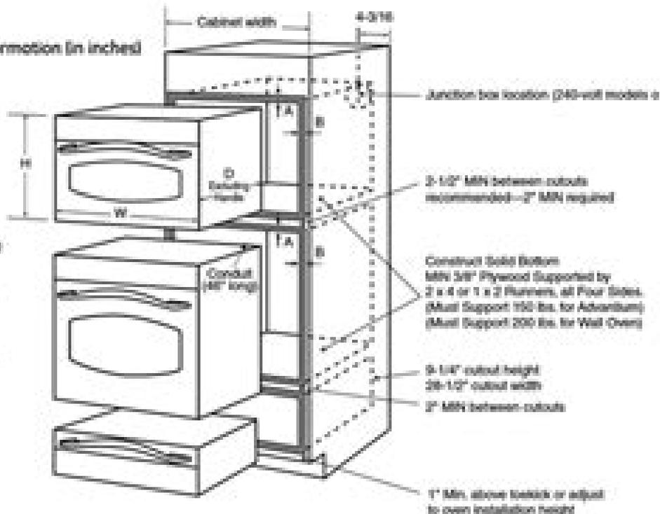
A=Allow 3/8" overlap of oven over bottom and 1/4" overlap at top edges of cutout.
