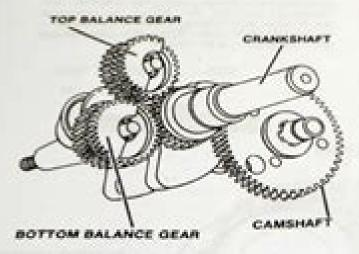
Figure 2 Components, Dynamic Balance System
