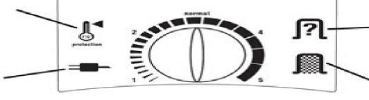
Bag Check - Should you attempt to operate cleaner without a filter bag, the unit will not start, and the bag check symbol will appear. Simply open the front cover and insert a new filter bag; the unit will then start.
