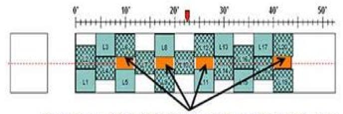
Four 2-ply 48"x 48" Air Bags Inflated to 2 PSI Max Along with 6" honeycomb void filler on each side of The air bag as shown in the photo.
