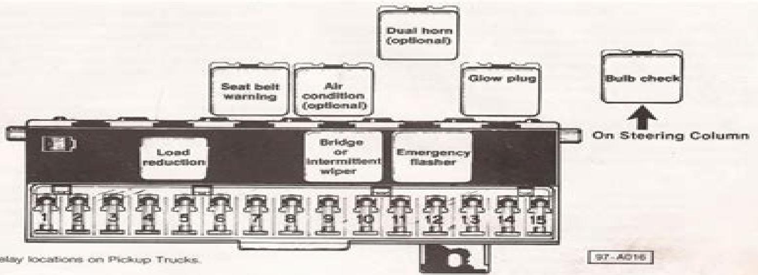
Fig. 12-5. Relay locations on Pickup Trucks.
