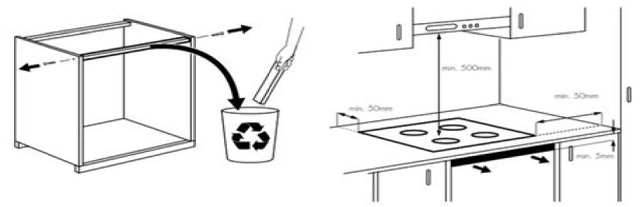
Make sure that a ventilation space of 5mm directly below the benchtop is included in the installation and kept the during use of the appliance. The warranty does not cover functional failures caused by the lack of an adequate ventilation space.
