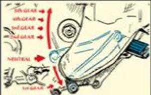
Shift to higher gears by pulling up on the gear shift with your foot. To shift down, push the gear shift down.
