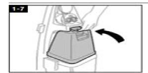
Replace clean solution tank (upper tank) by positioning bottom first. Press on tank handle to snap top of tank into place.
