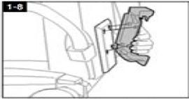
Attach tool holder Remove tool and taped screw from holder.
