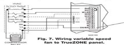
If using a Honeywell TrueZONE panel, the panel's DS/BK terminal is intended for use with a variable-speed fan. When one zone is calling (or less than 25% of capacity on systems with more than 4 zones), this terminal will be de-energized of 24 VAC. This reduces blower speed on most variable speed blowers.
