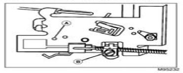
Hole in governor control lever must align with hole (A) in governor control plate.
