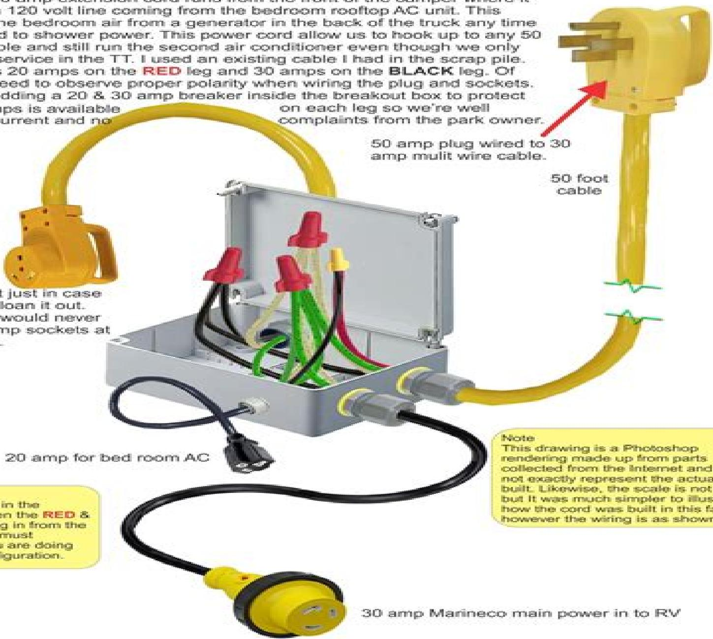
50 amp plug wired to 30 amp mult wire cable.
