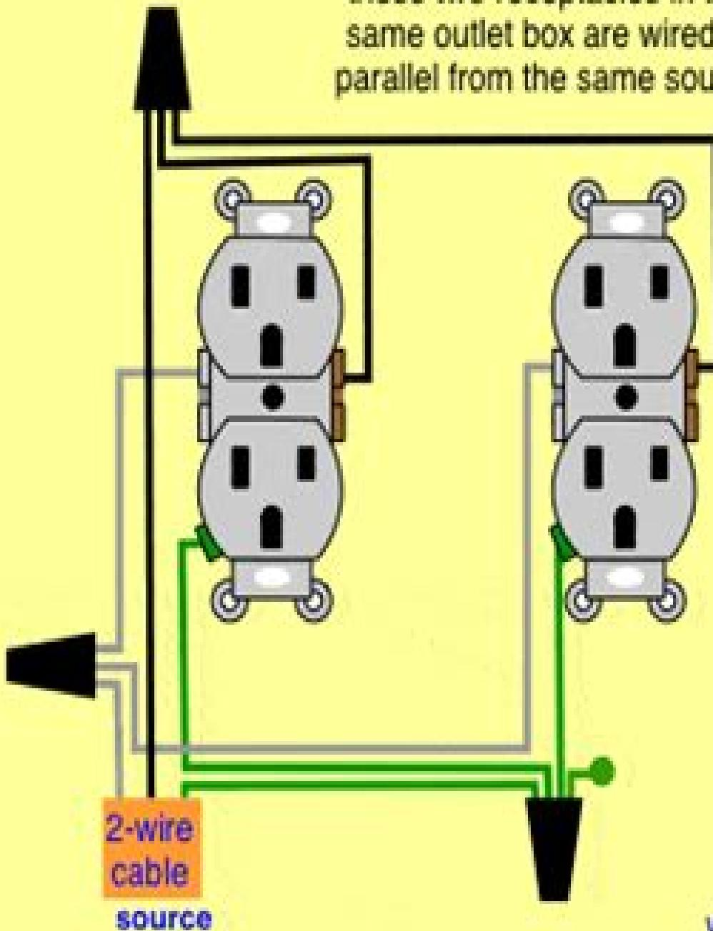
splicing the source to feed each receptacle separately allows either one to work even if the other one fails
