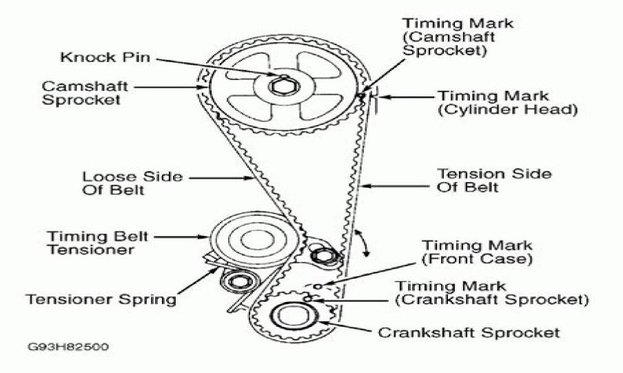
Fig. 1: Aligning Timing Marks
