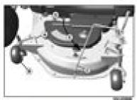
5. Potate at roser artirarap wheels to allow roser box. to be rolled outward away front machine:
