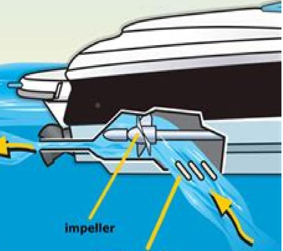
**intake grate:** Screening cover over the intake, which prevents large debris from entering
