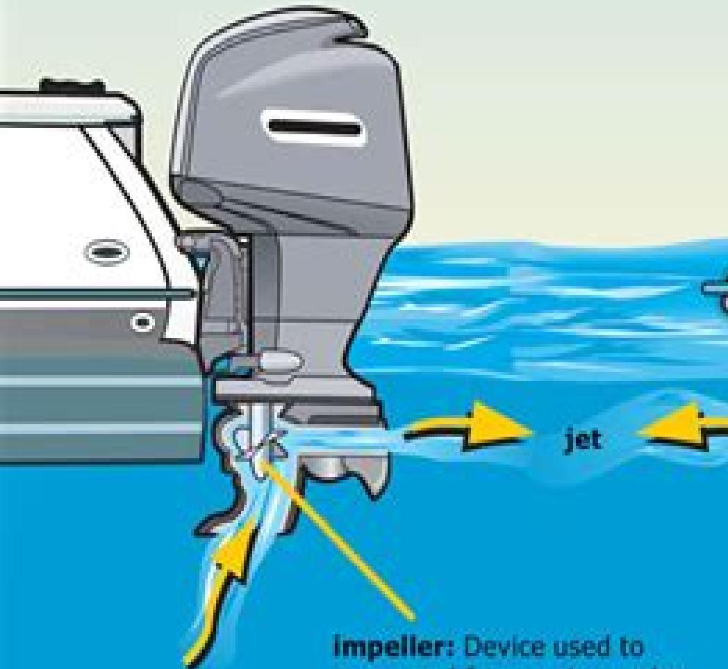
**intake:** Opening in the hull that draws water toward the impeller
