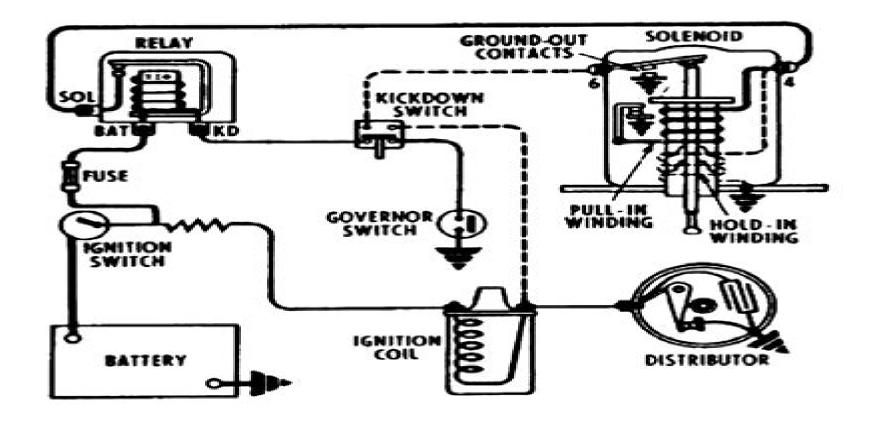
Overdrive Electrical Circuit Wiring Diagram
