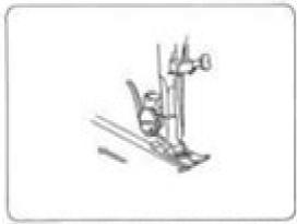
(3) Pull 15 cm (6") of both threads back and under the present foot.
