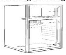
In the sidewalls of the refrigerator, there are four plastic sleeves with screws for securing the refrigerator. The sidewalls or rails attached for securing the refrigerator must be designed in such a way that the screws will remain firmly in place even when under increased load (while the vehicle is moving).
