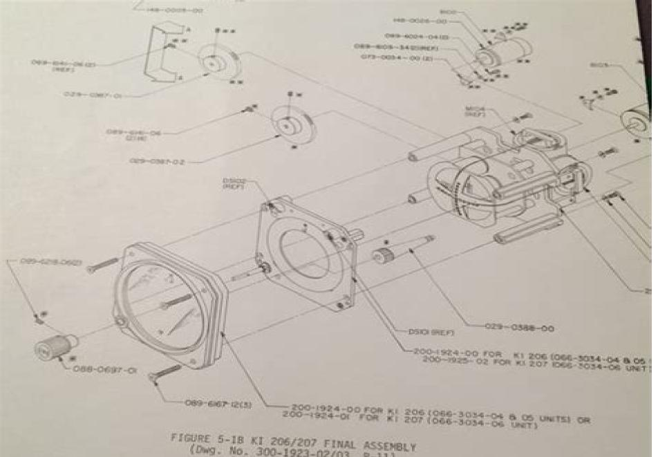
FIGURE 5-18 KI 206/207 FINAL ASSEMBLY (Dwg. No. 300-1923-02/03. R-11) (S/N Below 10.000) (Sheet 1 of 2)
