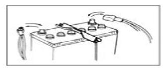
When removing the battery, we save to disconnect the negative cable first and then the positive cable. When reconnecting the battery, connect the positive cable first and then the negative cable, and replace the terminal cover.
