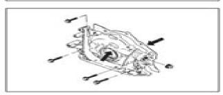
Whenever you use oil seals, gaskets, packing, O-rings, locking washers, split pins, self-locking nuts, and certain other parts as specified, be sure to use new ones. Also, before installing new gaskets, packing, etc., be sure to remove any residual material from the mating surfaces.
