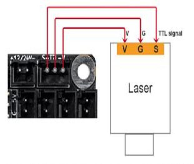
(V): V is the same as the power input, if the power input is 24V, then the output here is 24V. At present, the maximum power supported by the laser head is: 25W at 12V, and 50W at 24V.
