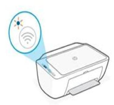
If the blue Wi-Fi light is not blinking, the printer might not be in Wi-Fi setup mode. Restart setup mode:
