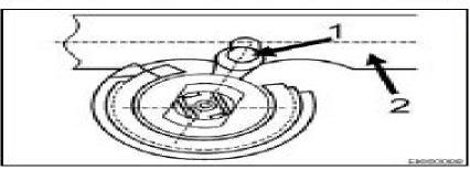
Turn the fuel injection pump control arm ( Item 1 ) to about centre position.
