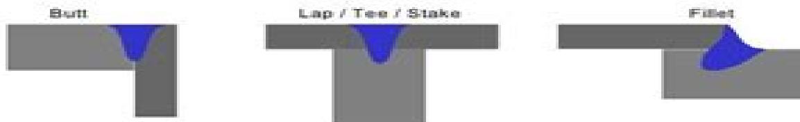
Figure G. Most common weld joints, most other types are variations on these.
