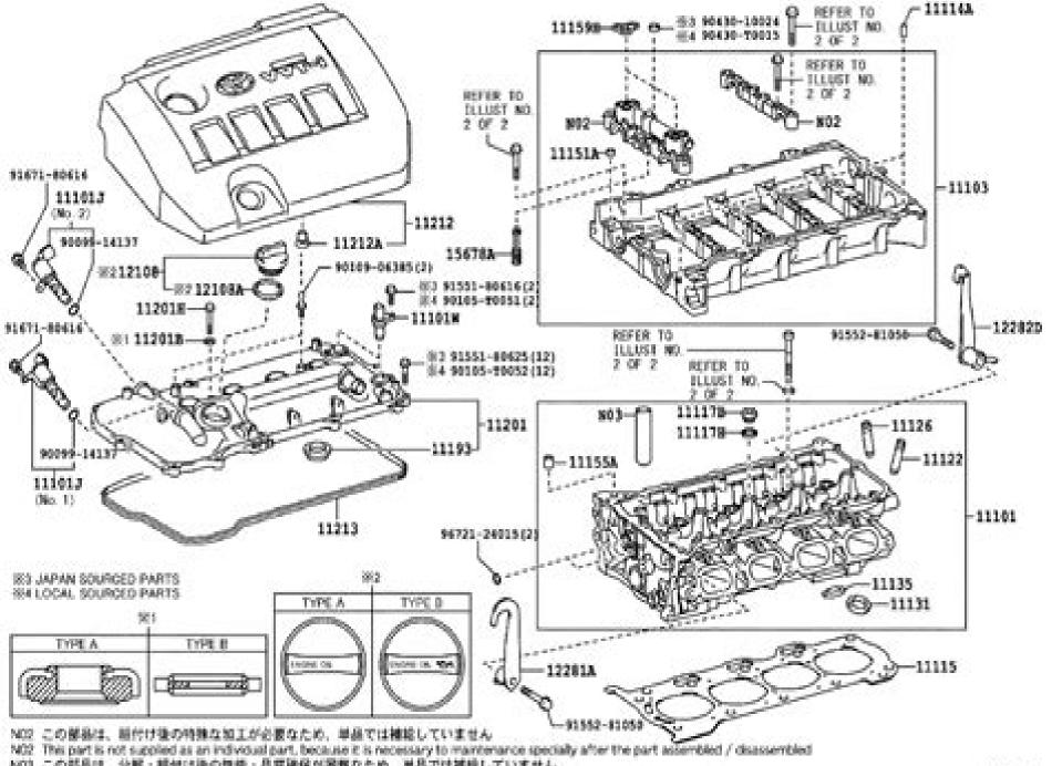
NO3. This part is not supplied as an individual part, because it is difficult to keep the function / quality of parts, assembled / disassembled
