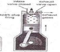
Piston pushes out burned gases.
