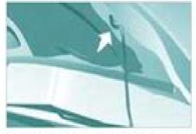
Secure the strut in one of the two notches, according to the height required, to hold the bonnet open.
