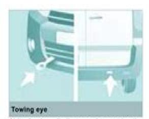
At the front, unclip the cover by pressing it at the bottom.
