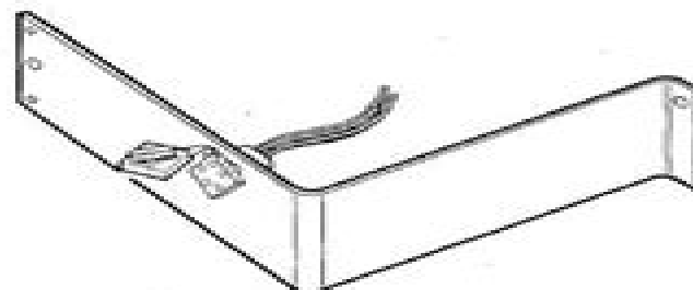
Fig. 2. Proper Installation of Female Receptacle Plug
