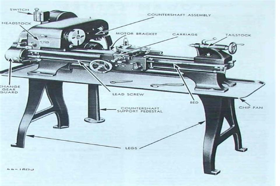
FIGURE 1-LOGAN FLOOR MODEL LATHE
