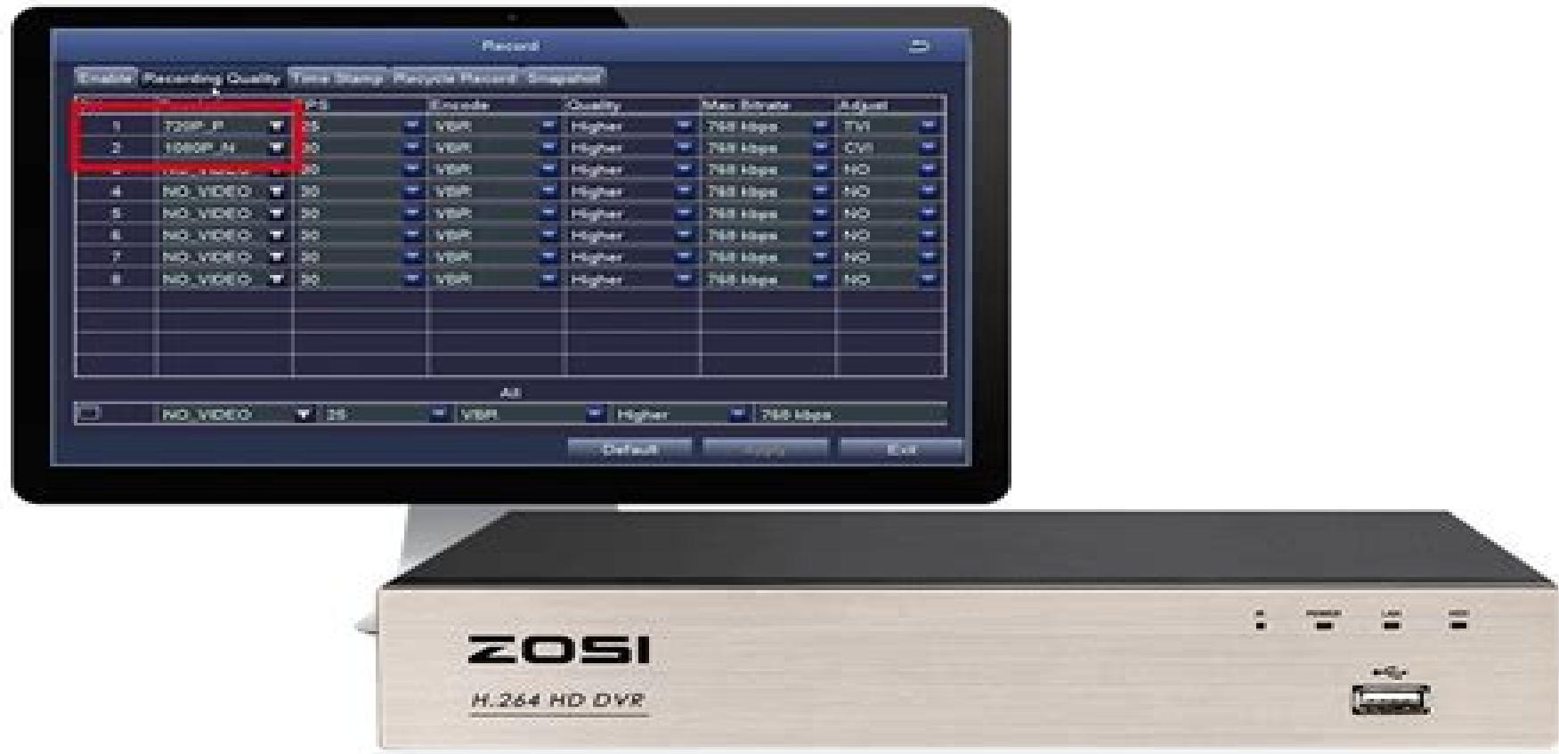
1. When it connect to 1080P Camera, the resolution is 1080P
