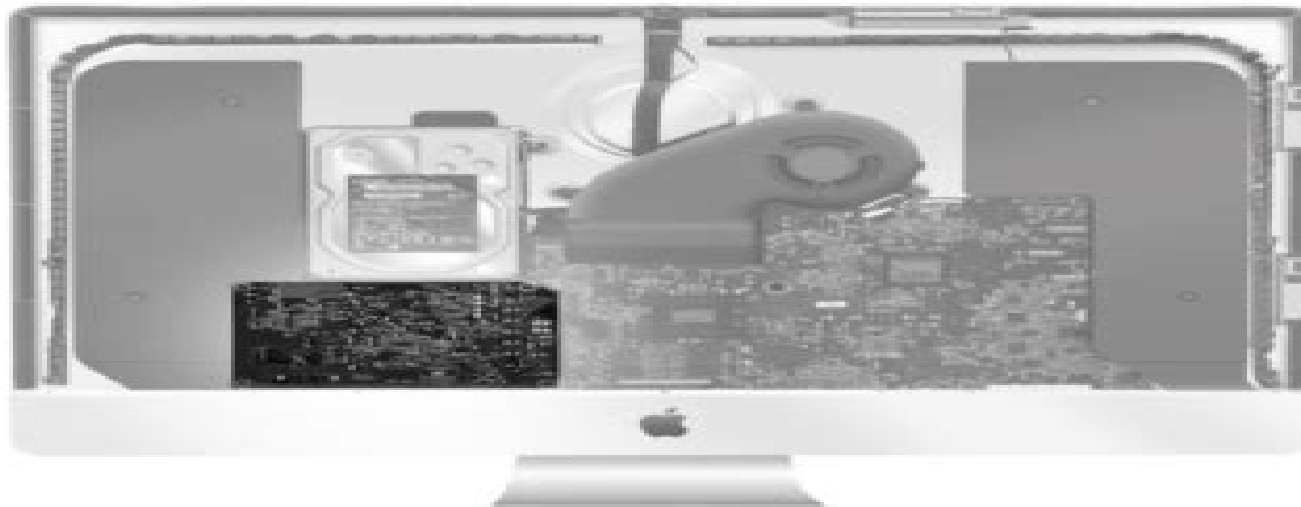
iMac (27-inch, Late 2012 – 2017): Logic board location
