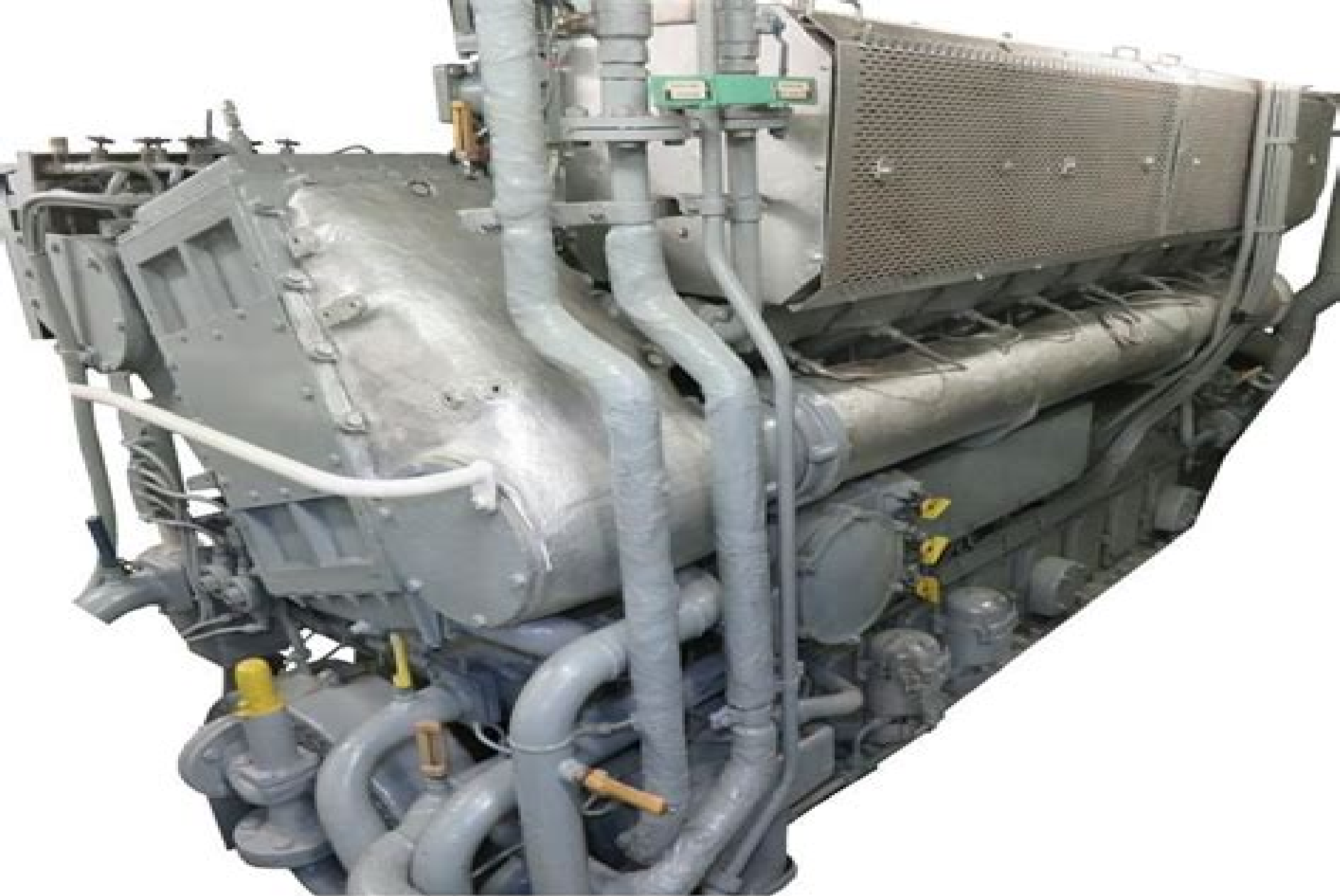
Deutz SBV 8 M 628 735 kW @ 684 RPM
