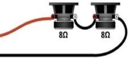
's connected in series add their impedance Ohms):  $8\Omega + 8\Omega = 16\Omega$
