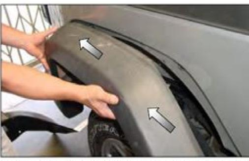
With all fasteners removed firmly take hold of the front lower edge of the flare and Pull up to release the mounting clips. You will hear a clicking sound as the clips are released. Continue to work your way towards the center then rear of the flare pulling firmly up and back on the flare as you go. Set the Factory Flare and Inner- liner on your work bench.
